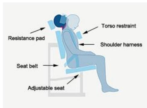
**Figure 5:** Cervical extension machine with several restraints
