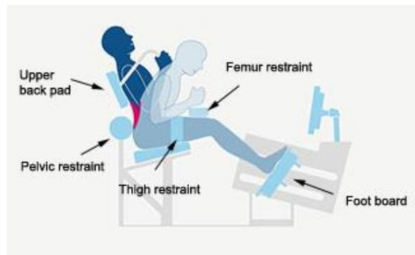
**Figure 4:** Lumbar extension machine with several restraints
